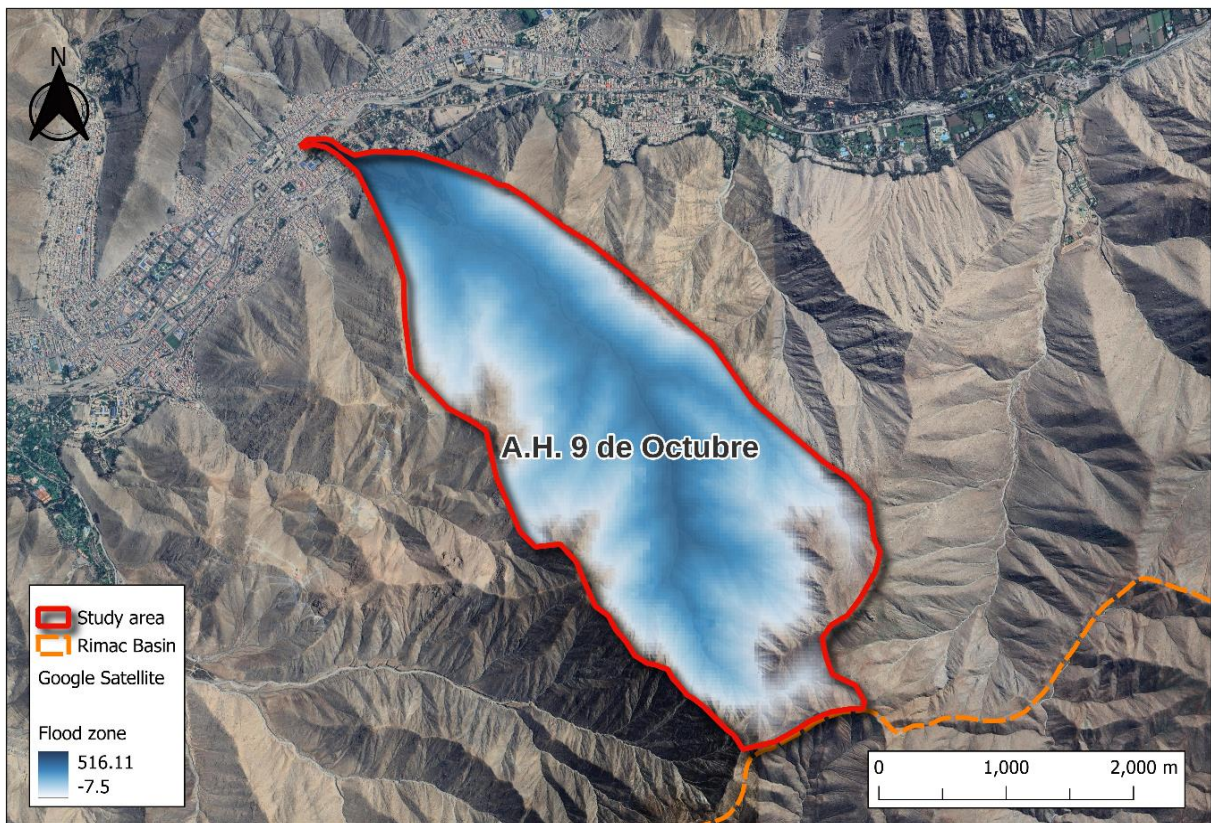
Figure 5. The humid zone according to the simulation for a flow rate of 61.2 m 3 /s, for a return period of 100 years
