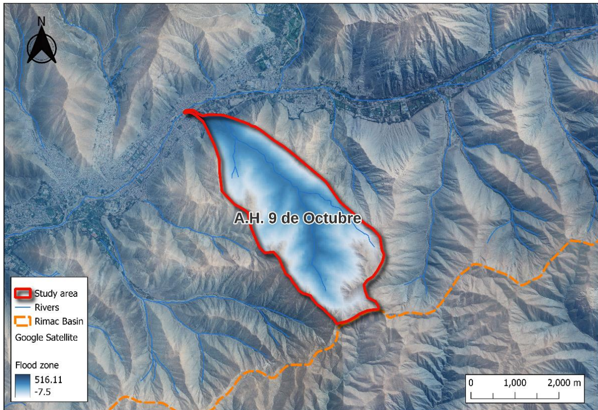
Figure 6. Simulation for a flow rate of 61.2 \text{ m}^3/\text{s} for a return period of 100 years
