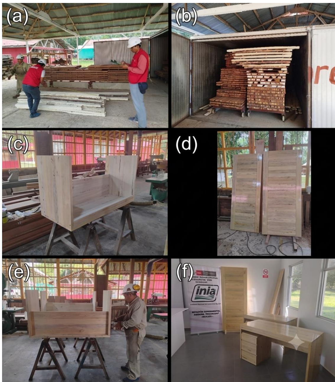
Figure 12. Production process of prototypes from thinning wood of Simarouba amara Aubl. Prototypes manufactured in the Carpentry Workshop of CITEforestal Pucallpa, Technological Institute of Production (ITP). (a) Determination of the initial volume ( m^3 ) of sawn wood. (b) Kiln drying of sawn wood in conventional drying chambers. The thicknesses processed were 1", 1.5", and 2". (c) Assembly process of components for the fabrication of a wooden desk. (d) Pre-finishing process of a solid wood door. (e) Application of the first coat of varnish on wooden desks. (f) Final presentation of the desk prototype (130 cm \times 60 cm \times 75 cm) and solid wood door (205 cm \times 83 cm), both finished using a sealed lacquer coating technique. The developed prototypes are currently exhibited at the Alexander von Humboldt Experimental Center, located in Padre Abad Province, Ucayali Region, Peru.
