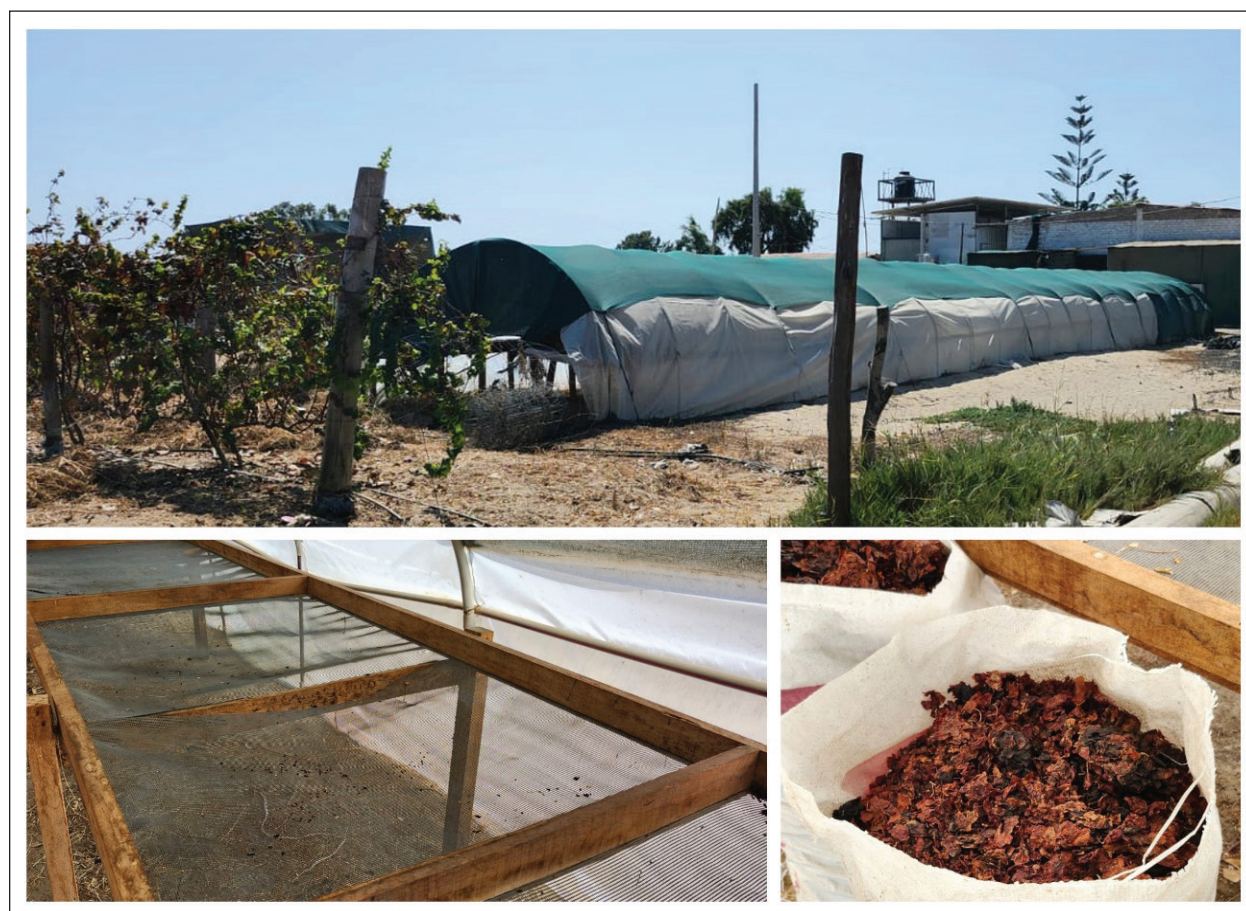
Fig. 2. Facilities for Quebranta grape pomace drying. Top: tunnel-type solar dryer tunnel; bottom left: trays for pomace drying; bottom right: dried grape pomace collected after 14 days in the trays.
