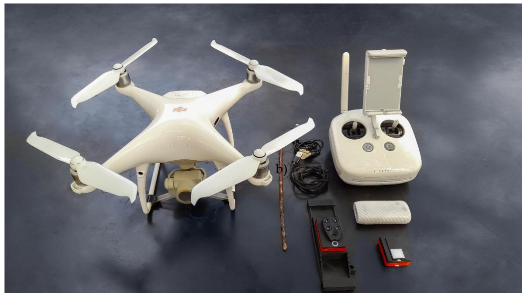
Figure 2. Equipment used in data collection. RPAS and radio control, and Parrot Sequoia camera.
