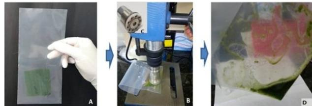
**Figure 1.** A: Plastic bag (20 x 10 x 0.01cm) used for the bench drill maceration with banana leaf sample (5 x 5 cm); B: Bench drill maceration of the sample in the plastic bag with 2 mL of extraction not, maceration buffer; C: Biorema drill (Agdia<sup>®</sup>); D: Macerated leaf sample with extraction buffer.
